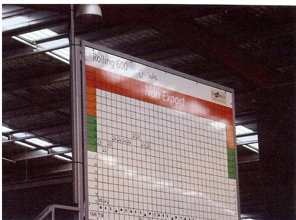
Visual management – quality control (rolling 600) boards are located on each packing line.
